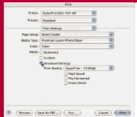
In the Macintosh Interface, a pull-down menu provides access to Print Settings, which include Media Type, Print Quality and High Speed. The same pull-down menu accesses Printer Color Management controls, where you can turn off the printer's color adjustment.
