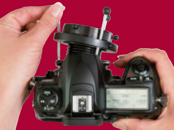
Fine adjustments to the position of the sweet spot are made by adjusting the focusing post knobs.
