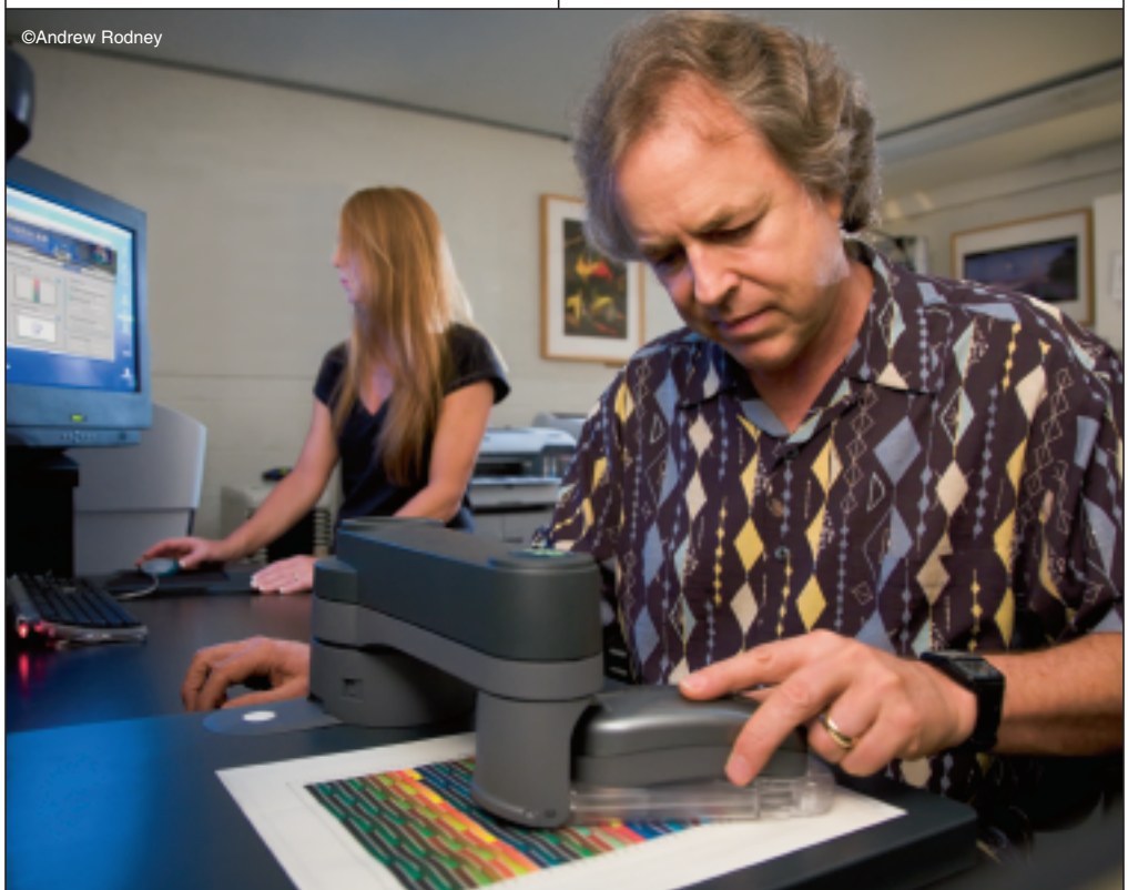
Mac Holbert sets up the Eye-One iO to measure a target for building a custom ICC paper profile.
