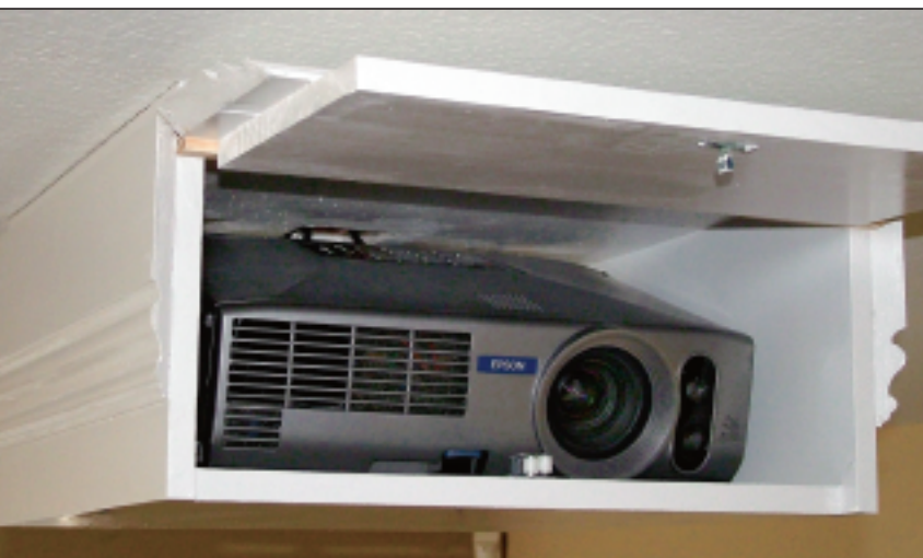
I house the Epson 835p projector in a custom-built box with easy access to both the front and the back, which is mounted to the ceiling.
