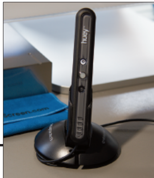
Figure 1. The huey sits in a holder near the display, periodically measuring and making adjustments for the ambient light conditions.
