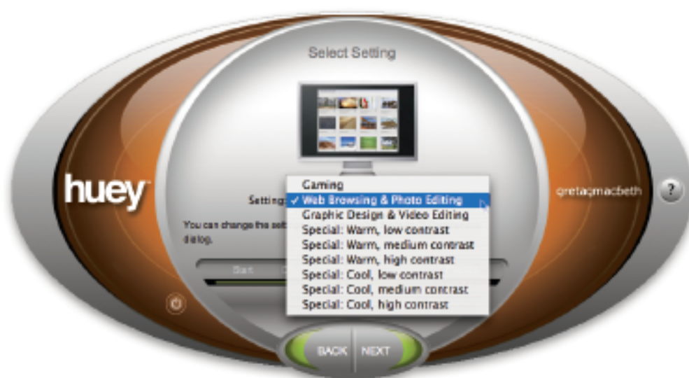
Figure 4. The available color settings correlate to the following target values: Cool = 7500K, Medium = 6500K, Warm = 5000K, Low contrast = 1.8, Medium contrast = 2.2, High contrast = 2.5.
