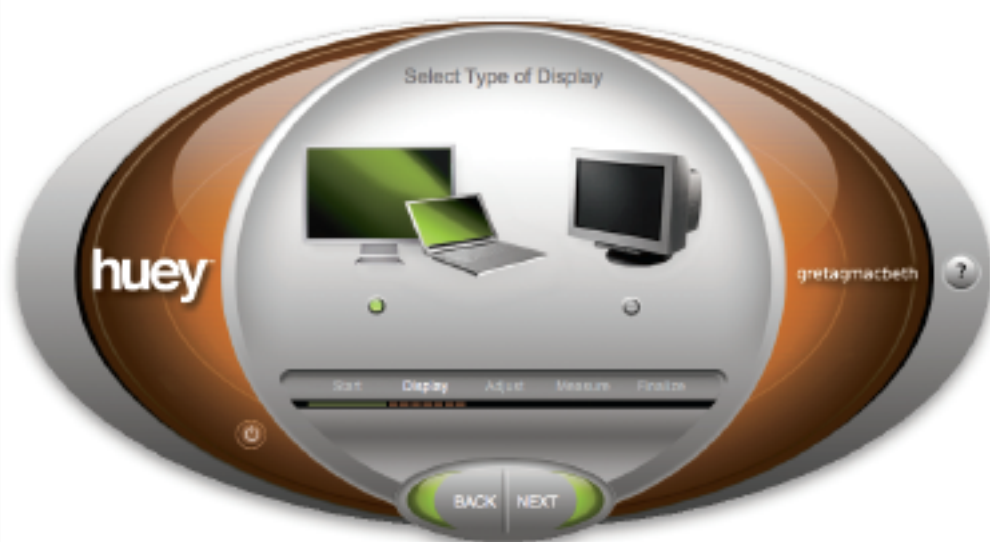
Figure 2. The user interface is a modern design devoid of excess elements to confuse the novice user. Here you choose the type of display and click the Next button. All the steps are outlined in a simple status bar at the bottom so you always know where you are in the process.
