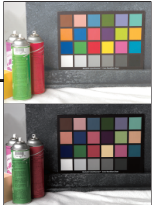
The darker image above was shot in linear mode with no processing to render it to output referred. The image at top is output referred for ColorMatch RGB, which is based on the behavior of a calibrated CRT display.
