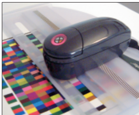
The X-Rite Pulse (DTP20) has audible and visual alerts to indicate the results of the measurement. The red light ring means there's an error; green would indicate success.
