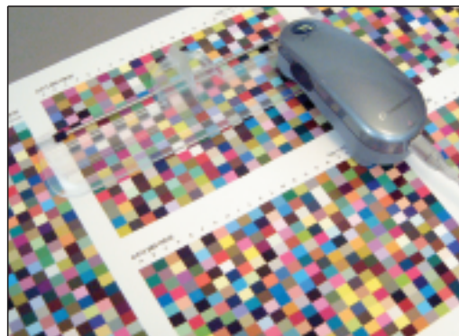
The ECI2002 chart is available as four letter-sized documents or two large pages. This is a letter-sized chart. The GMB Eye-One has a small plastic guide to use as you drag the Eye-One device across the chart. Notice how the charts are randomized to assist in color patch recognition.
