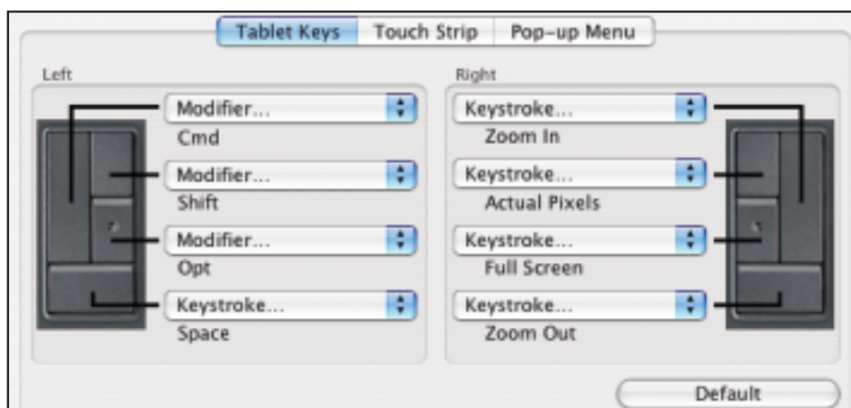
The Intuos3 driver allows you to customize each of the keys on each side of the tablet. You can choose what works best for your work style.
