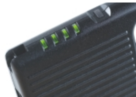
When you press the test button with no load on the unit, green indicator lights show the level of charge remaining. Four green indicates full charge.
