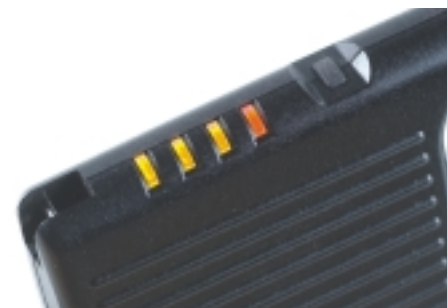
With a load on the unit, orange and red indicator lights show the level of charge remaining. Three orange lights and one red indicate full charge. As power is consumed, the orange lights flash to indicate the depletion.
